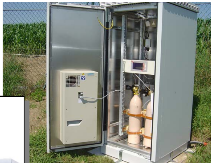
Ambiant CH 4 analysis Based on MGA3000 analyser CH 4 analysis Indoor or Outdoor Cabinet with gas sampling
