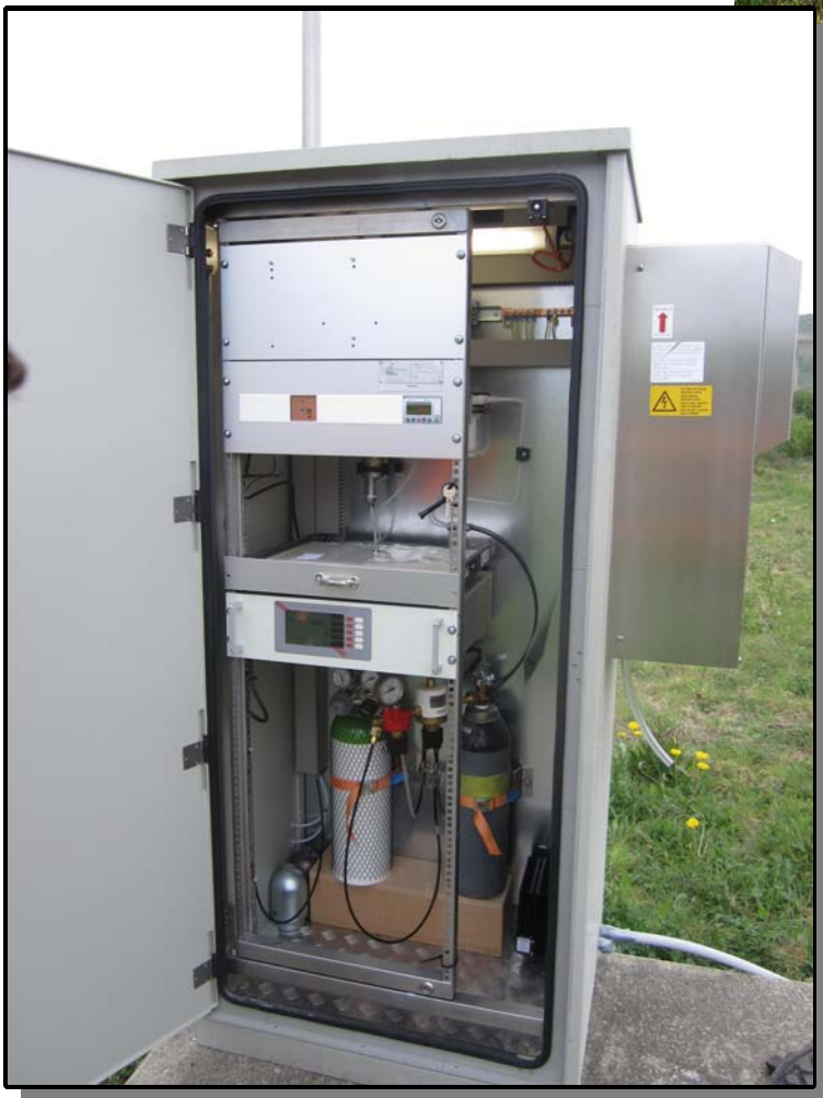
Ambiant CH 4 analysis Based on MGA3000 analyser CH 4 analysis Indoor or Outdoor Cabinet with gas sampling
