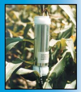
SGB16 sap flow sensor with weather shield attached.
