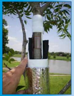
EXO Sensor showing the different layers of insulation and shielding that comes with each sensor.
